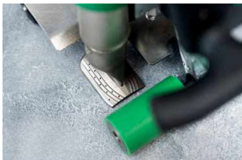
Simultaneous butt welding on seam tape
